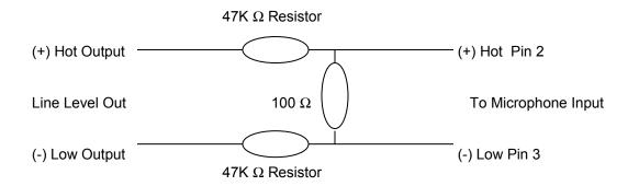
The 3 resistors used above are 1/4 to 1/8 watt <u>metal film</u> at <u>1%</u> precision.
